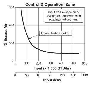
**NOTE:** Input at low fire changes with ratio regulator adjustment.
